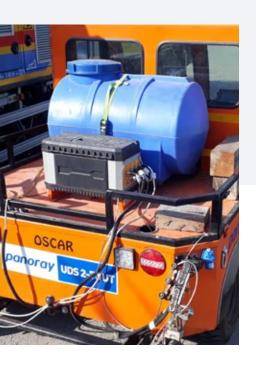
Ultrasonic inspections of the 1,100 km line according to EN 16729 standard with the railway vehicle which can be measured with 10 km/h measurement speed and their manual verification
